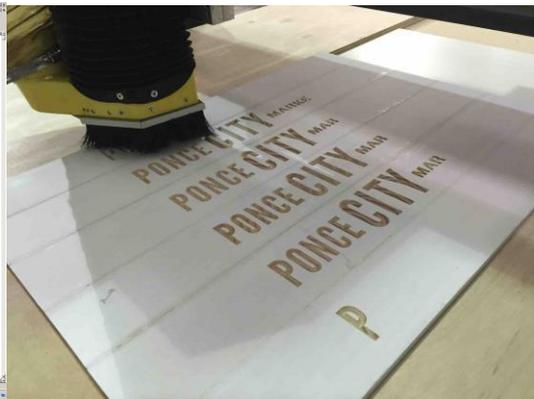
After the router had finished its work, the faces and side panels were glazed and painted black. All the pieces were then assembled to create the A-frame signs.
